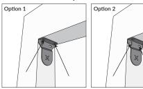
Holding the bracket in place flush with front of opening, mark the mounting screw locations in the top of the bracket (option 1) or the side of the bracket (option 2) with a pencil. Pre-drill marked locations using a 1/8 in. drill bit. Attach the brackets using the supplied mounting screws and a Phillips screwdriver.
