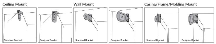
Fit the shade into the brackets and center the shade over the window (this may take two people). With a pencil, mark the wall on the side of one bracket. Remove the shade and then attach the one bracket with two screws, Next, insert the shade into the second bracket. Hold the shade up and insert other end into the already mounted bracket, making sure that the shade is level. Mark the wall on the side of the second bracket. Remove the shade and install second bracket with two screws.
