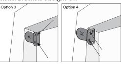
Holding the bracket in place mark the mounting screw locations in the side of the bracket (option 3) or the back of the bracket (option 4) with a pencil. Pre-drill marked locations using a 1/8 in. drill bit. Attach the brackets securely using the supplied mounting screws and a Phillips screwdriver.
