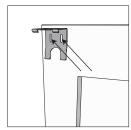
Remove the brackets from the headrail assembly. Align each bracket with your location marks and while holding the bracket in place, mark the mounting screw locations in the back of the bracket with a pencil. Pre-drill marked locations using a 1/8 in. drill bit. Attach the brackets securely using the supplied mounting screws and a Phillips screwdriver.
