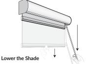
To lower the shade, pull down on the weight bar and release or pull down on the wand then release. Repeat until the desired position is reached.
