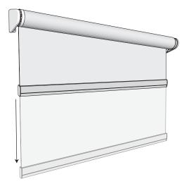
**1B:** With one hand hold the shade roll and the other hand firmly holding the tensioner device, carefully push the tensioner upwards on the bracket (1) then push the entire shade roll to the right (2) (or left depending on your installation configuration) until you can cleanly remove the shade roll from the shade roll hanging bracket
