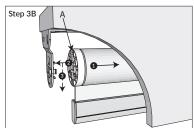
**3B:** With the arrow of the tensioner (A) pointing upward, push the pin end towards its bracket, depressing the pin (1), align and insert the hooks of the left bracket into the tensioner device (2), then gently pull down on the shade until the hooks have locked securely to the tensioner (3).
