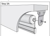
**3A:** While firmly holding the tension device and shade roll, align the center and the 4 small pins of the spring loaded pin end of the shade roll and insert into the holes of the shade roll hanging bracket.
